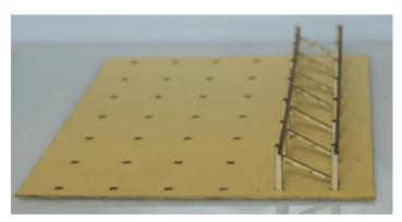
Step 3: Glue the cross braces in place as shown.
