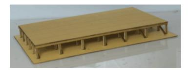
Step 6: Position and glue the platform decking in place.
